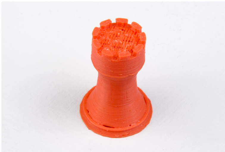
Figure 3.11: An example of insufficient top layers.
